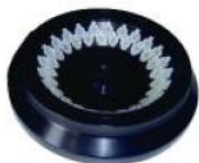
R-5 Capacity:48x0.5ml Max speed:13000rpm Max RCF:19910xg Adapter:48x0.2ml
