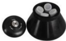
R-14 Capacity:4x100ml Max speed:10000rpm Max RCF:13280xg Adapter:4x0.2ml Adapter:4x5ml Adapter:4x20ml Adapter:4x0.5ml Adapter:4x10ml Adapter:4x30ml Adapter:4x1.5/2.2ml Adapter:4x15ml Adapter:4x50ml
