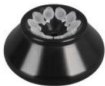
R-9 Capacity:10x5ml Max speed:14000rpm Max RCF:13610xg Adapter:10x0.2ml Adapter:10x0.5ml Adapter:10x1.5/2.2ml
